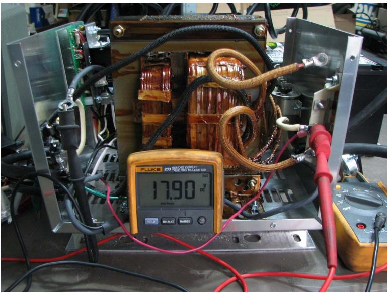
Capacitor Disconnected, Batteries Disconnected. DC Voltmeter Verify the Connections have been removed from the Capacitor
