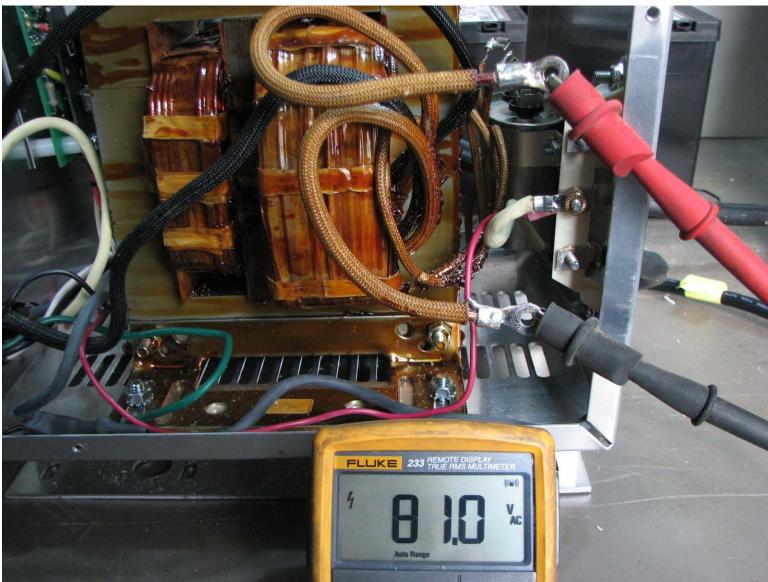
Capacitor and Batteries Disconnected AC Voltmeter
