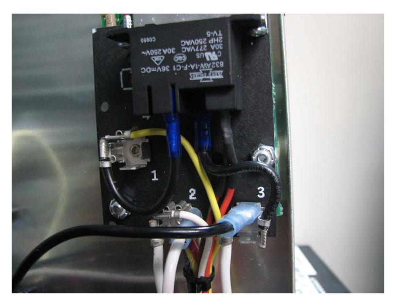
2) By simply removing the wire from Pin 1 and connecting it to Pin 3. Pin 1 remember, is coming from the AC Line Power HOT.
