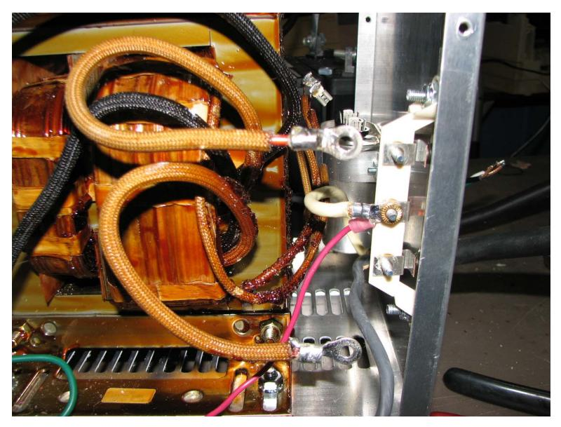
Use Insulated Pliers to remove the connectors at the Capacitor. Capacitors can store a charge for an extended period of time. Caution should be taken when working on or around Capacitors.
