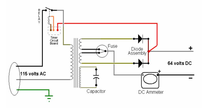
This is a simplified schematic and represents all Lestronic II Battery Chargers. Make a diligent effort to trace the wiring in the charger and become familiar with the routing and components.
