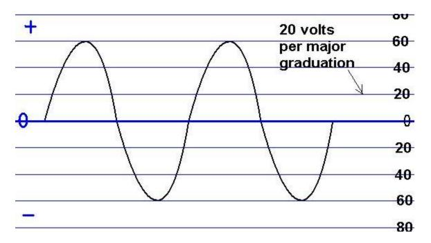
The scope is displaying a value of approximately 60 AC Volts Peak. The voltmeter in previous photos is displaying the 40.5 volt RMS values.
