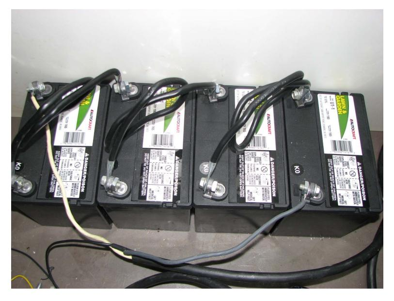
These are Lawn and Garden Tractor batteries. They are 12 volts each wired together in series to total 48 volts. These batteries will be adequate for testing purposes only.
