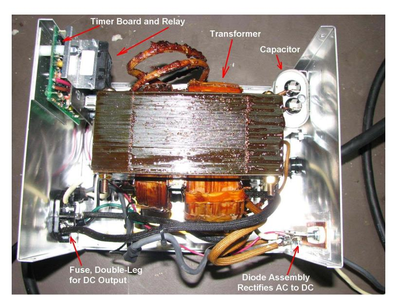
Take the time to Locate and Identify all the Components inside the Battery Charger.
