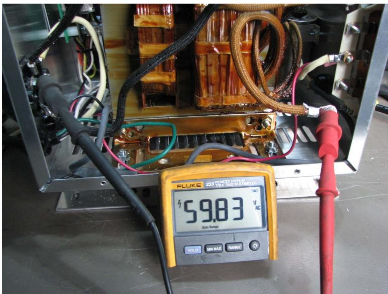
Capacitor Connected, Batteries Disconnected. AC Voltmeter
