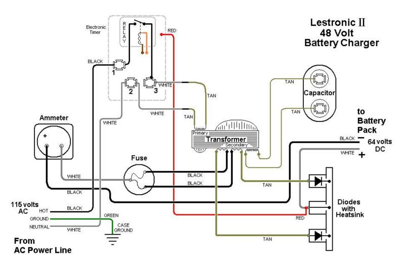
The two low voltage SECONDARY WINDINGS have their voltage directed to the BATTERIES through the two DIODES when their potential is positive. When one TAN wire from the low voltage secondary is positive, the other TAN wire on the other low voltage secondary is negative. Each coil and diode set up a Half Wave Rectifier. The polarities of the low voltage secondarys reverse each time the AC signal reverses (50 or 60Hz).
