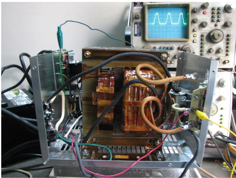
Half Wave Rectification with only Coil 2 attached to Diodes Capacitor NOT Connected
