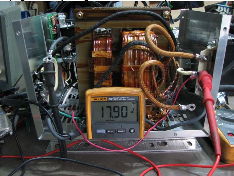
Capacitor Disconnected, Batteries Disconnected. DC Voltmeter Carefully remove the Connections at the Capacitor and insulate. Plug the Battery Charger into the AC mains power line.
