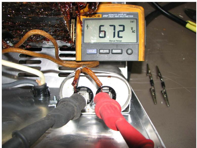
**Connect Capacitor, Leave Batteries Disconnected.** AC Voltmeter Carefully connect the Secondary Coil Windings to the Capacitor using Insulated Handle Pliers.
