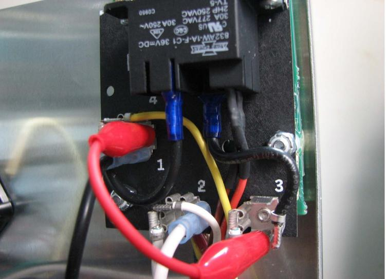
1) By Jumping a wire from Pin 1 to Pin 3 This in effect bypasses the Relay.
