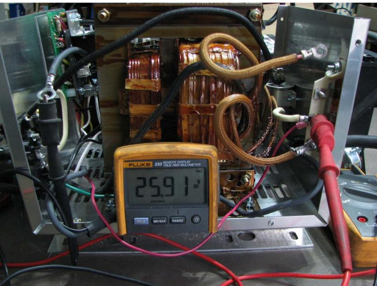
Capacitor Connected, Batteries Disconnected. DC Voltmeter
