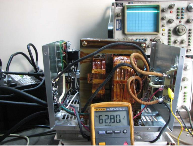
Capacitor Connected, Batteries Connected, Secondary Connected to Diode Assembly, AC Power Cord Plugged In DC Voltmeter
