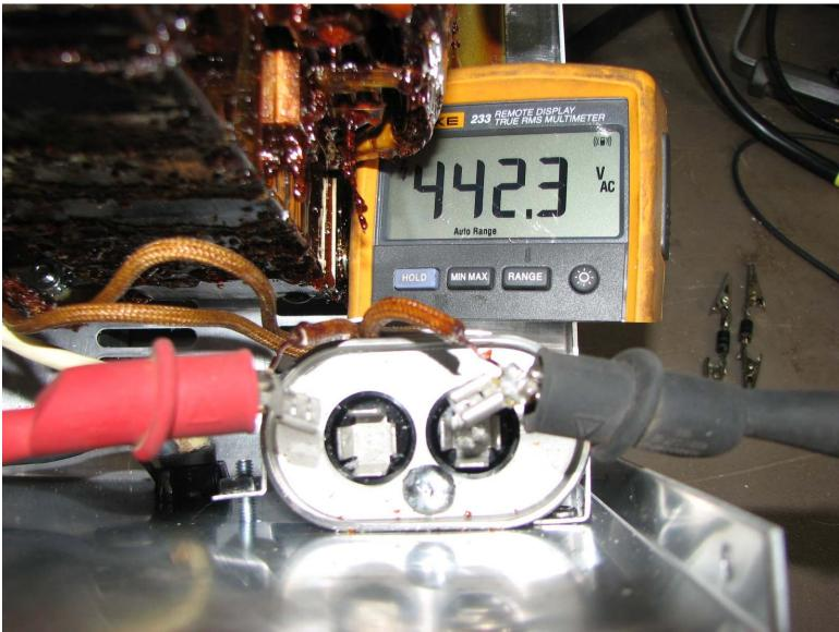
Capacitor and Batteries Disconnected AC Voltmeter
