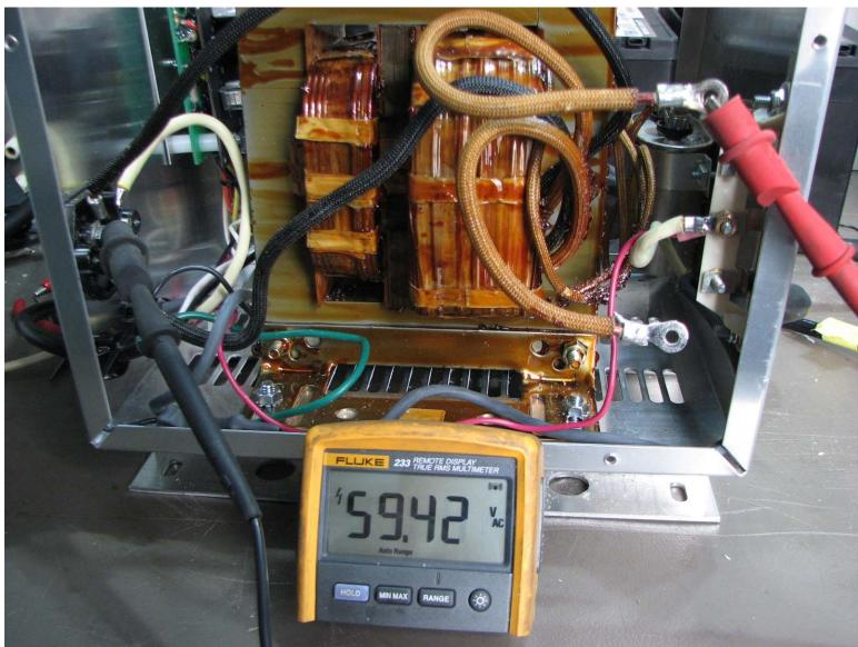
Capacitor Connected, Batteries Disconnected. AC Voltmeter
