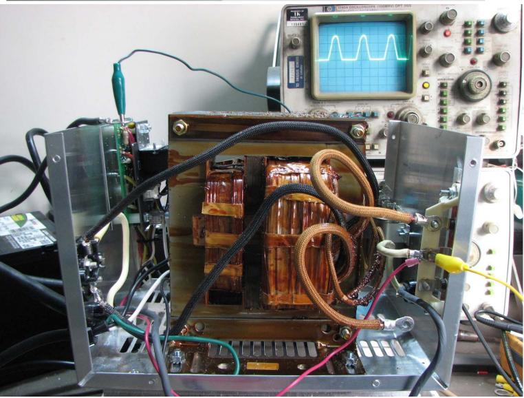
Half Wave Rectification with only Coil 1 attached to Diodes Capacitor NOT Connected
