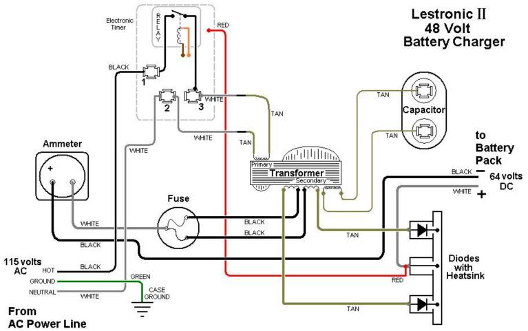
When the AC Power Cord is plugged into a live receptacle and the DC Power Output is connected to a known good 48 volt DC set of batteries, the battery voltage will follow the RED wire from the DIODE ASSEMBLY to the ELECTRONIC TIMER CARD.
