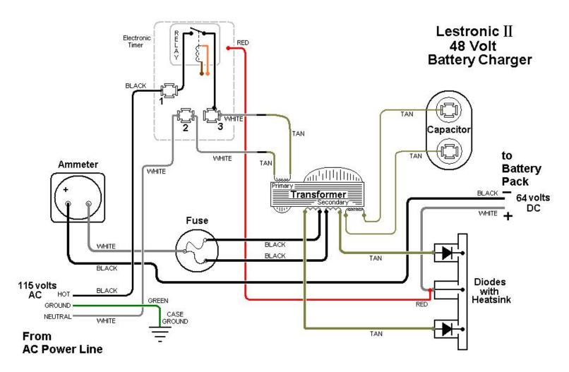
2.1 volts per battery cell is considered a fully charged wet lead acid battery.There are 24 battery cells in a 48 Volt DC Battery System.That will total to 50.4 volts DC for a fully charged 48 volt system
