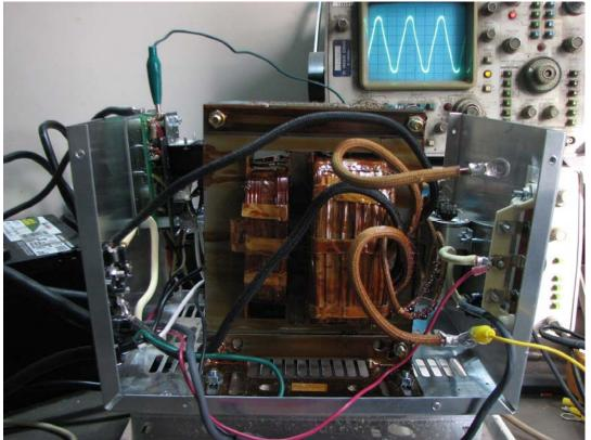
This photo shows AC pattern at output of lower Secondary Coil Coil #2
