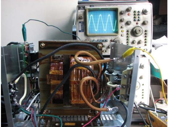
Top photo shows AC pattern at output of upper Secondary Coil Coil #1
