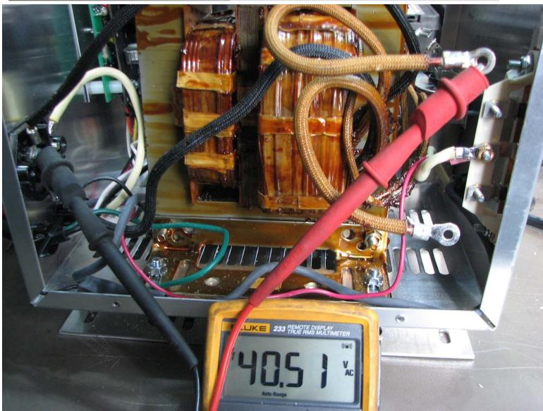
**Next: Capacitor and Batteries Disconnected AC Voltmeter** Connect the Voltmeter leads to the Charger Negative (here shown at the Fuse) and the Coil Lead from the Secondary Winding as shown in this photo. For the sake of this discussion we will label this lead **Coil #1**.
