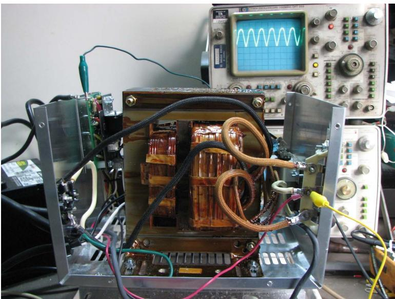
Full Wave Rectification with AC Signal being fed through both 1 and 2 Coils Capacitor NOT Connected
