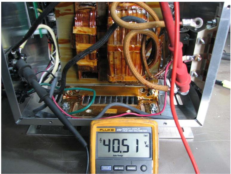
Capacitor and Batteries Disconnected AC Voltmeter
