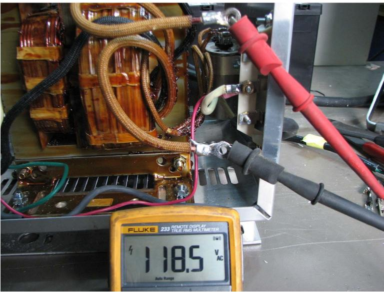
Capacitor Connected, Batteries Disconnected. AC Voltmeter
