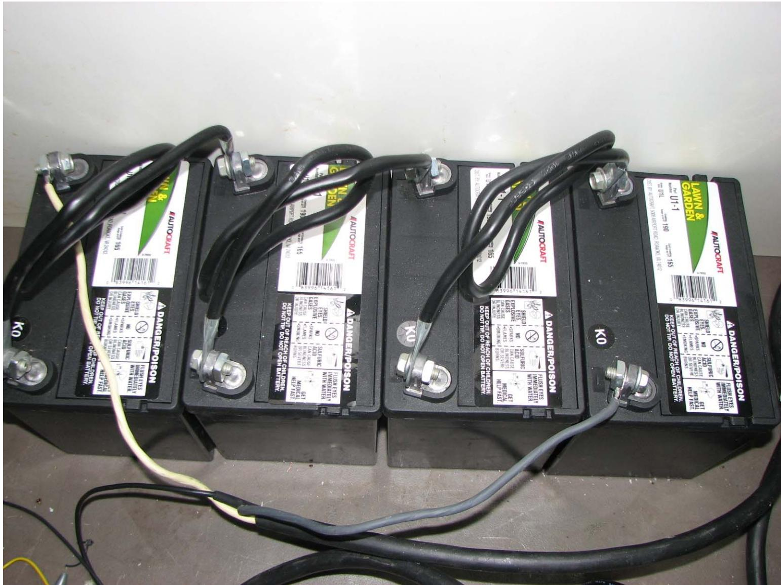
These are Lawn and Garden Tractor batteries. They are 12 volts each wired together in series to total 48 volts. These batteries will be adequate for testing purposes only.
