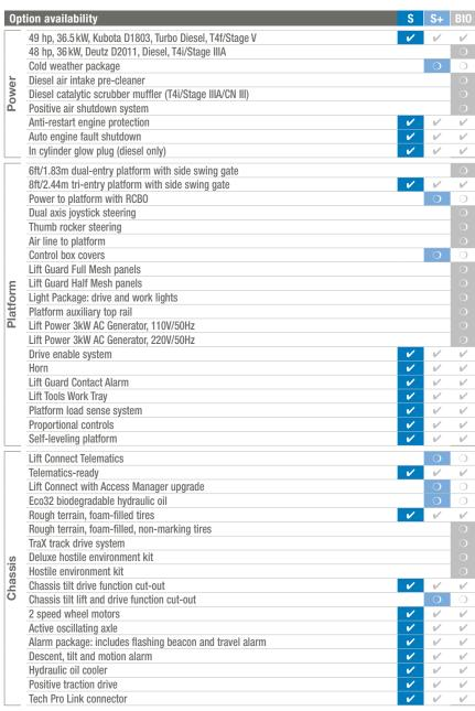
Cold weather package not available on Kubota engine Positive air shutdown system for Kubota engine only
