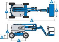
\* The metric equivalent of working height adds 2 m to platform height. U.S. adds 6 ft to platform height. \*\* In lift mode (platform raised), the machine is designed to operate on firm, level surfaces only. \*\*\* Gradeability applies to driving on slopes. See operator's manual for details regarding slope ratings.
