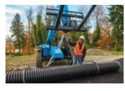
All Genie telehandlers come equipped with a lift shackle that enable you to sling a load without secondary attachments. A factory lift shackle lift chart provides clear capacity limitations to the operator.
