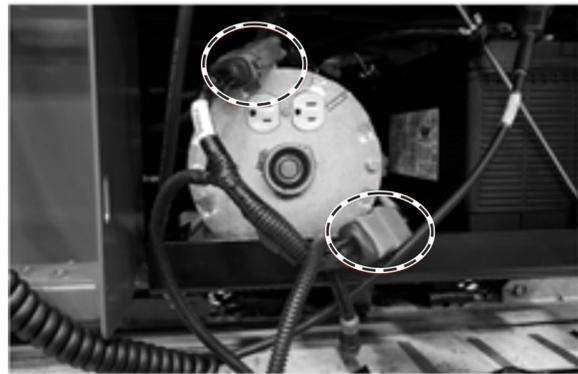
Note: Harness connectors are keyed for proper installation.
