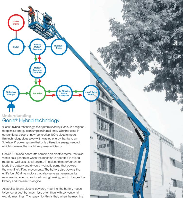
As applies to any electric-powered machine, the battery needs to be recharged, but much less often than with conventional electric machines. The reason for this is that, when the machine is operated in hybrid mode, the diesel engine automatically takes over from the battery when the level of charge declines, driving the hydraulic pump directly and recharging the batteries.
