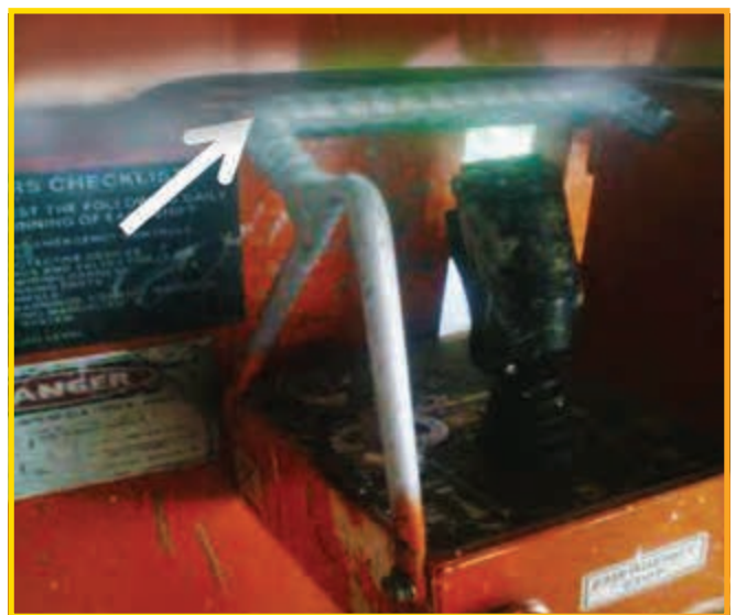
FIG1: Unauthorised 'Adhoc' guard (arrowed) welded above manufacturers original guard may cause scissor lift to become unstable if hoses, leads etc. become snagged on it.
